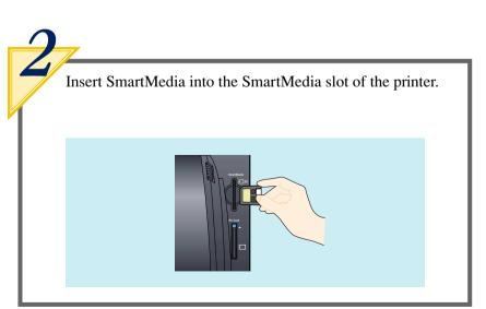
Insert SmartMedia all the way into the printer.
